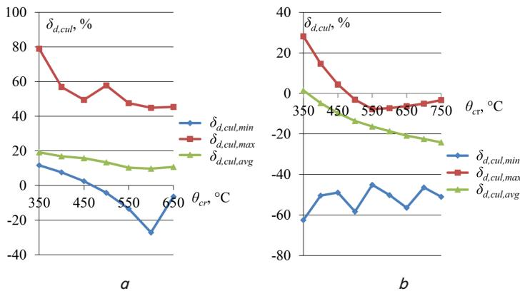
Fig. 3. Dependences of  $\delta_{d,cul,min}$  minimum value,  $\delta_{d,cul,max}$  maximum value and  $\delta_{d,cul,avg}$  average value on the critical temperature of steel: a – for the reactive fire-protective material; b – for the passive fire-protective material
