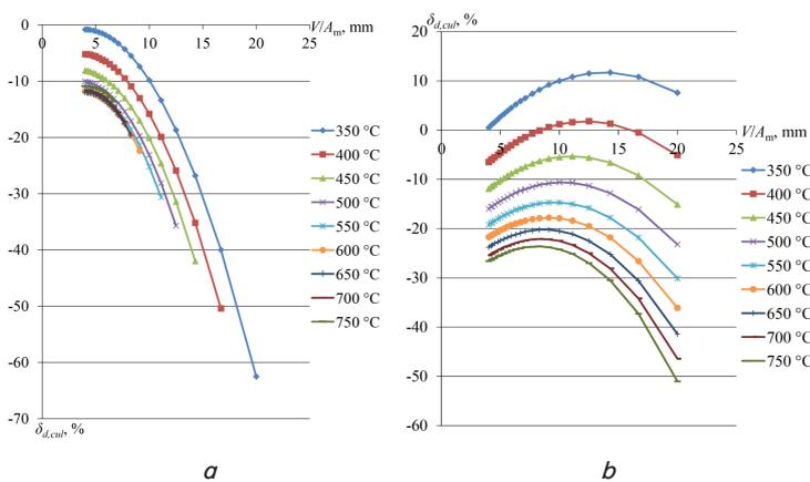
Fig. 2. Dependence of  $\delta_{d,cul}$  deviation on  $V/A_m$  reduced thickness defined for the passive fire-protective material: **a** – for the normalized fire resistance threshold of 60 minutes and different values of  $\theta_{cr}$  critical temperature ( $^{\circ}\text{C}$ ); **b** – for the normalized threshold of fire resistance of 150 minutes and different values of  $\theta_{cr}$  critical temperature ( $^{\circ}\text{C}$ )
