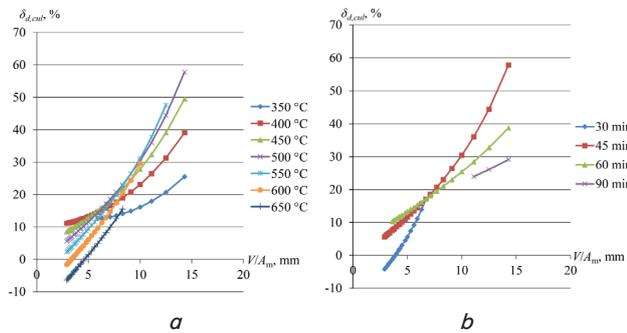
Fig. 1. Dependence of  $\delta_{d,cul}$  deviation on  $V/A_m$  reduced thickness defined for the reactive fire-protective material: **a** – for the normalized threshold of fire resistance of 45 minutes and different values of  $\theta_{cr}$  critical temperature of steel ( $^{\circ}\text{C}$ ); **b** – for the critical temperature of steel of  $500\text{ }^{\circ}\text{C}$  and different values of  $t_{cr}$  normalized fire resistance threshold (min)
