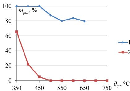
Fig. 4. Dependence of  $m_{pos}$  positive values of  $\delta_{d,cul}$  deviation on the critical temperature of steel: 1 – for the reactive fire-protective material; 2 – for the passive fire-protective material
