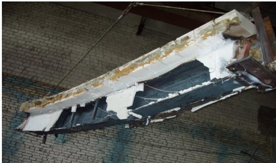
Fig. 6. Physical appearance of a loaded beam with the passive fire-protective material after the test
